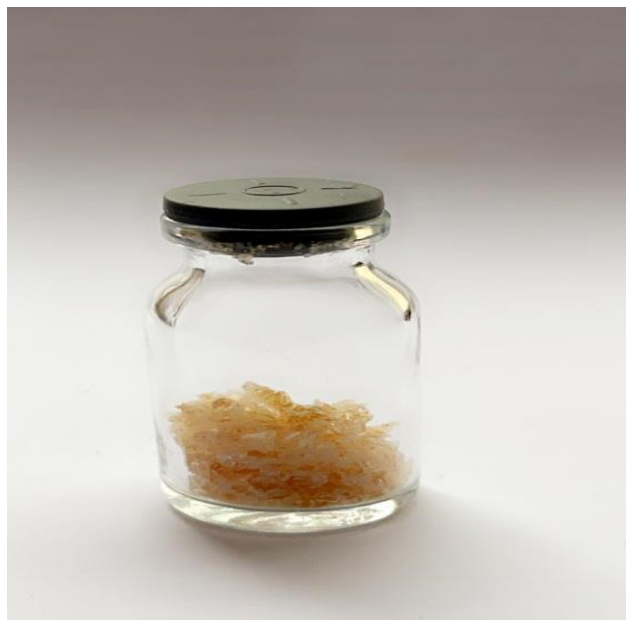
Figure 3. Image of a sample of the hybridized solid hybrid polymer (EMA-co-TMSPMA-co-HPMA)
