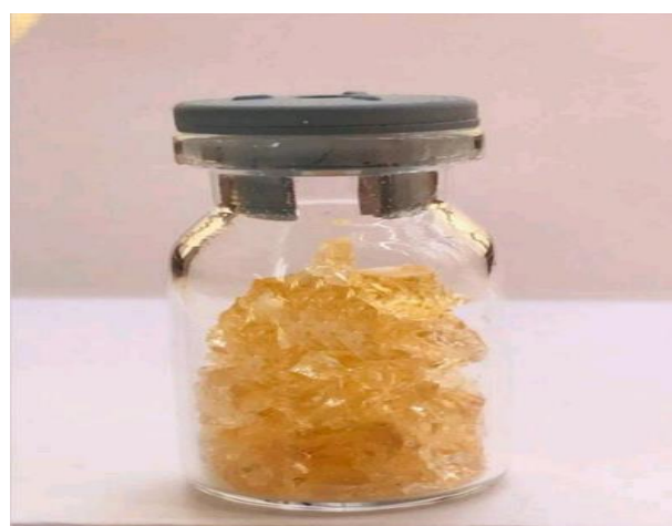
Figure (2) the dried hybridized packed sample for the solid hybridized polymer (iso-BMA-b-TMSPMA-b-HPMA).
